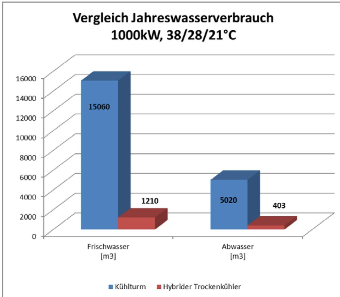
*Water consumption of a cooling tower compared to that of a hybrid cooler of an example system for year-round full-load operation and constant cooling power of 1,000 kW with fluid temperatures of 38/28°C in Munich*
