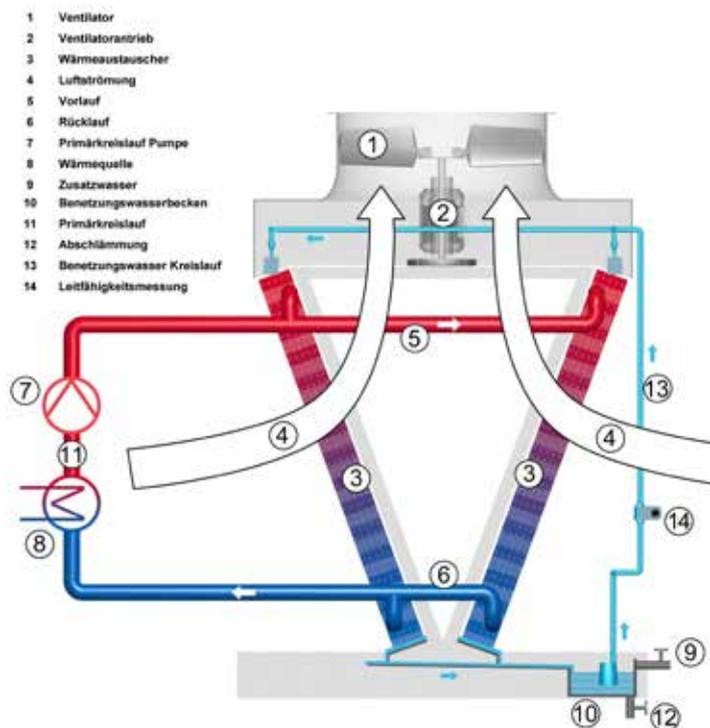
Function diagram of the hybrid dry cooler, JAEGGI Hybridtechnologie AG
