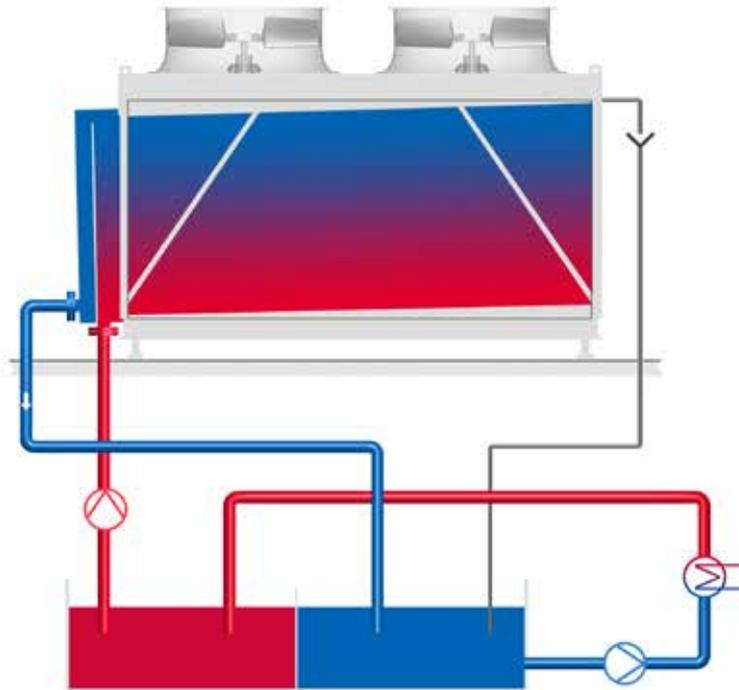
*Function diagram for dry cooler system with cooling water and self-draining hybrid cooler*
