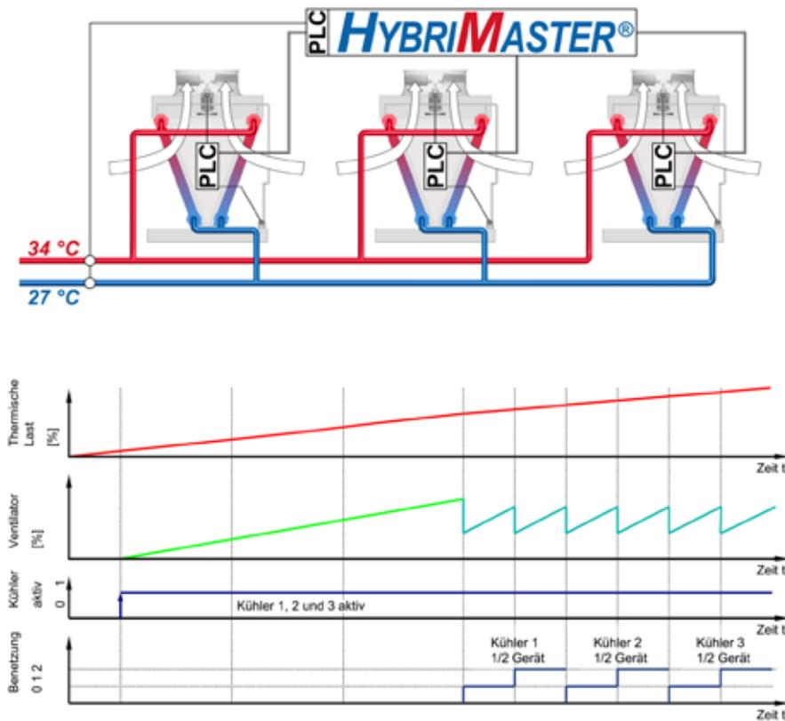
Master-slave control principle in compound systems with several hybrid coolers
