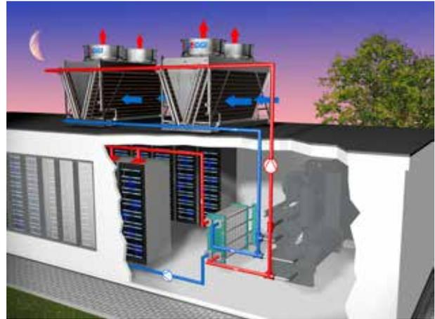
*Example of a data centre application with “free cooling”. The chiller operates only at high wet bulb temperatures. In the normal operating mode, the chiller is bypassed and only the hybrid coolers are used.*
